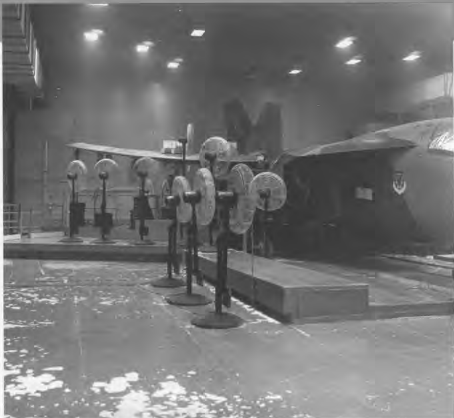
To verify the structural integrity of critical components, F-111s are chilled to minus 40 degrees while the wings are subjected to a simulated 7.33 g.
