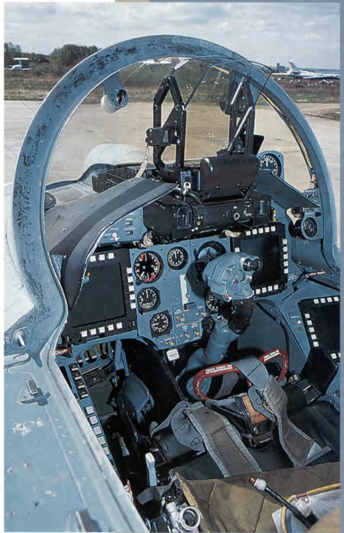
The Su-35's cockpit contains a large head-up display and a number of multifunction display screens.
