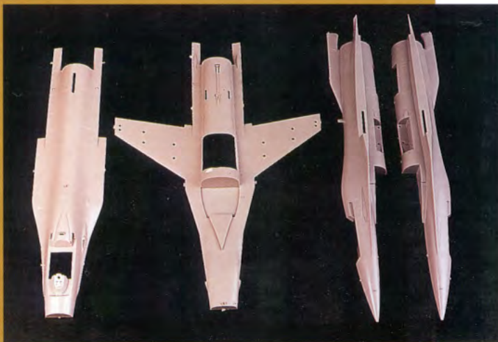
Most manufacturers split the F-16 fuselage into top and bottom halves for molding (left). Tamiya is one of the few companies that chose to split the fuselage into left and right halves (right).
