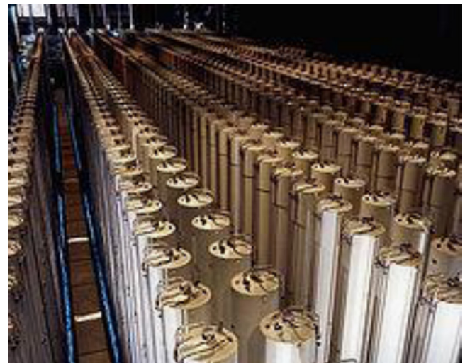
Fig. 7. Cascade of gas centrifuges. Piketon Ohio 1984.
