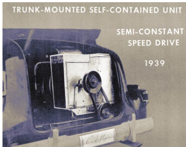
Figure 2: The self-contained automotive air conditioner installed in the trunk of a 1939 Cadillac.
