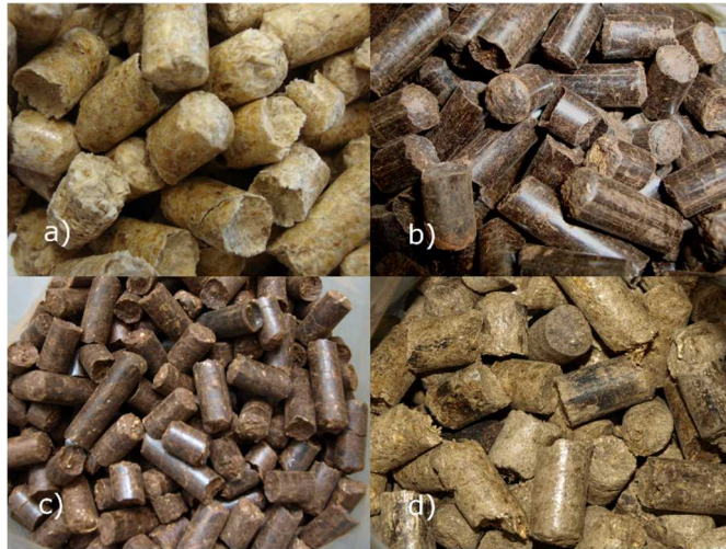
Figure 1. Examples of pellets made from different raw materials: a) commercial wood pellet, b) peat pellet, c) a mixture of pine bark and peat and d) rye straw pellet.
