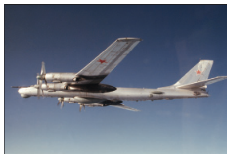
Tu-95RTs Bear D targeting platform with Uspekh / Big Bulge X-band radar located under the centre section.
