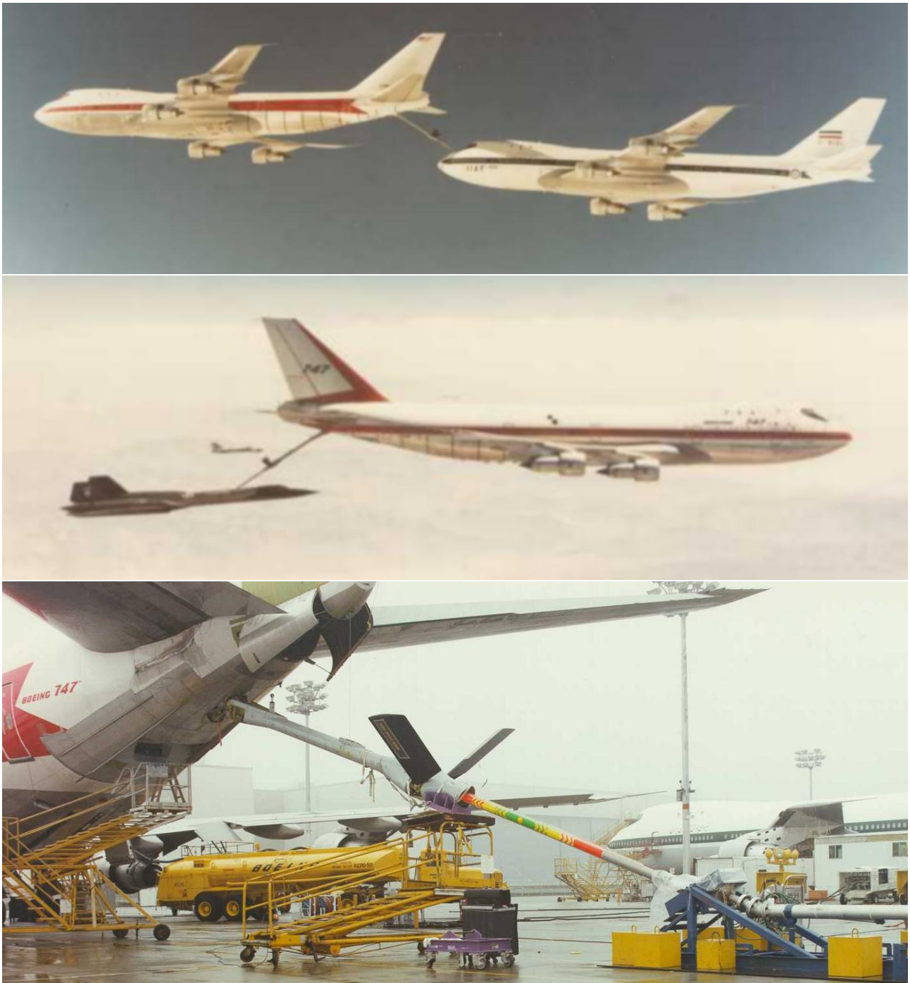
Figure 8: The Boeing 747-400 represents the best value for money aerial refuelling tanker available, moreso if mothballed late model 747-400 airframes are used. The 747-400 is a low risk option, since a number of 747 tanker conversions were performed during the late 1970s (US Air Force).
