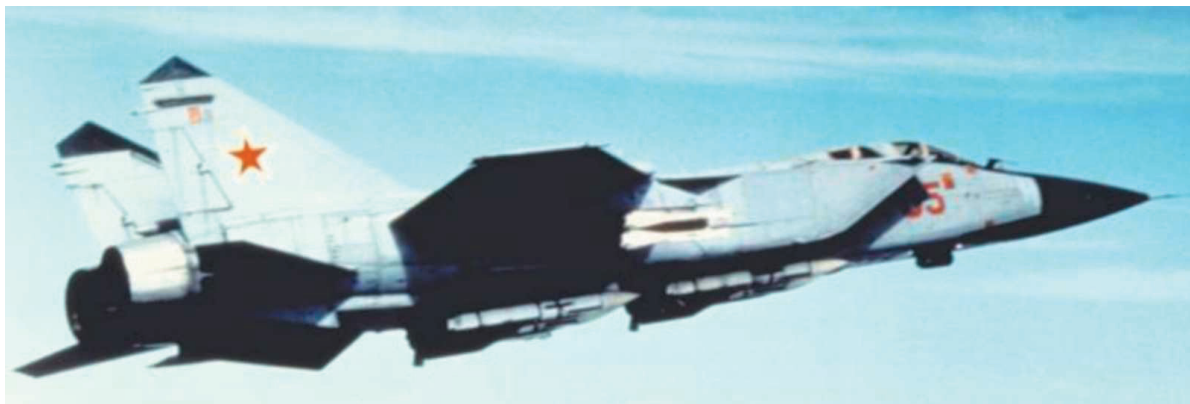
The only two fighters ever specifically built for cruise missile/bomber defence were the Russian MiG-31P Foxhound (above) and US Navy F-111B (below). The MiG-31P was built to kill B-52s and B-1s, and the F-111B the Backfire. These airframes are nearly identical in cardinal weight/size parameters, built to carry large look-down/shoot-down radars,IRST systems and similar R-33/AA-9 and AIM-54 missiles. (US DoD)
