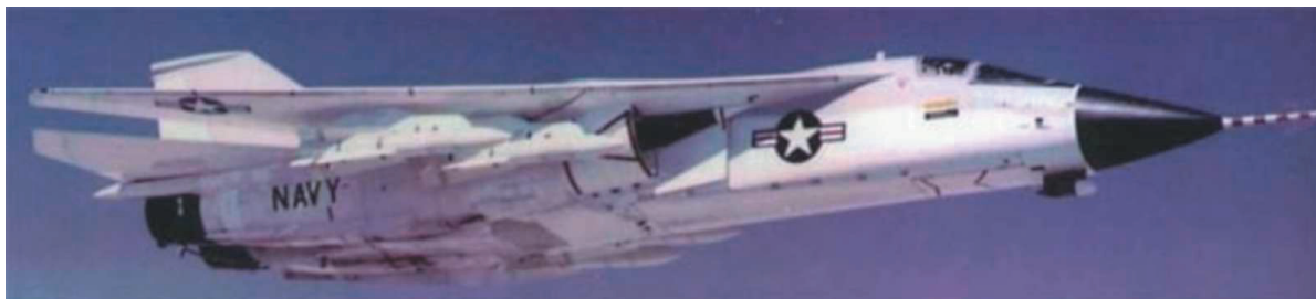
The only two fighters ever specifically built for cruise missile/bomber defence were the Russian MiG-31P Foxhound (above) and US Navy F-111B (below). The MiG-31P was built to kill B-52s and B-1s, and the F-111B the Backfire. These airframes are nearly identical in cardinal weight/size parameters, built to carry large look-down/shoot-down radars,IRST systems and similar R-33/AA-9 and AIM-54 missiles. (US DoD)
