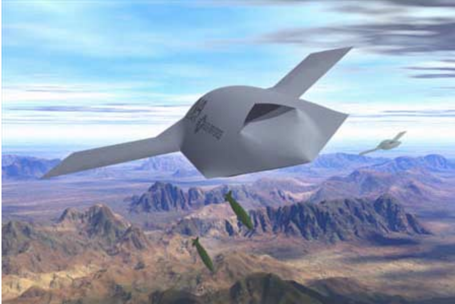
Figure 6. Boeing/DARPA UCAV demonstrator, here depicted dropping a pair of GBU-32 JDAM GPS/inertial guided bombs (Boeing).
