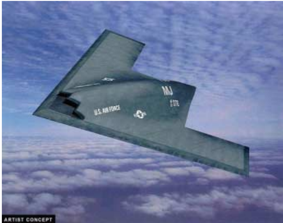
Figure 7. Northrop-Grumman UCAV Proposal. This design evidently exploits the low observable design rules devised for the B-2 bomber (Northrop-Grumman).
