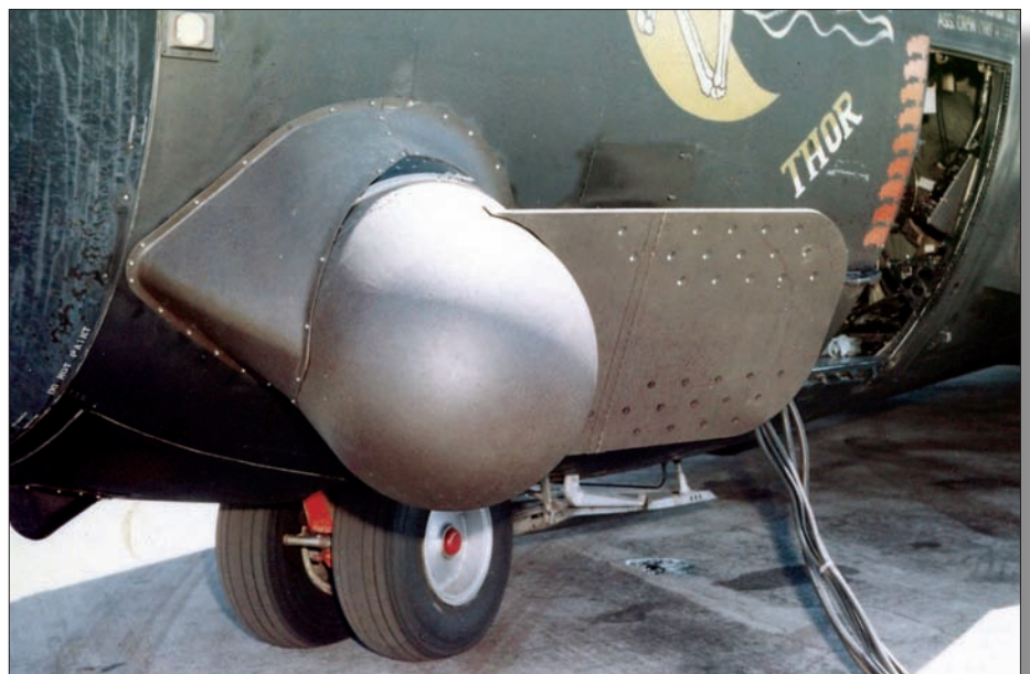
The ASD-5 Black Crow sensor was fitted to many reconnaissance and interdiction aircraft, including this AC-130A Surprise Package gunship. It could track ground vehicles using the radio emissions from their ignition systems.
