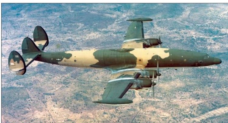
The EC-121R Batcats were radio relay platforms, which collected signals from ADSID sensors and relayed them via a steerable X-band datalink to the ISC at Nakhon Phanom.
