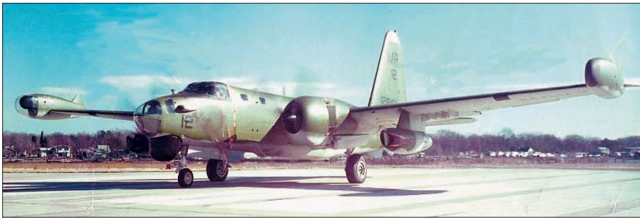
The OP-2E was a heavily modified P-2V Neptune used to deliver ADSIDs along the Ho Chi Minh Trail.
