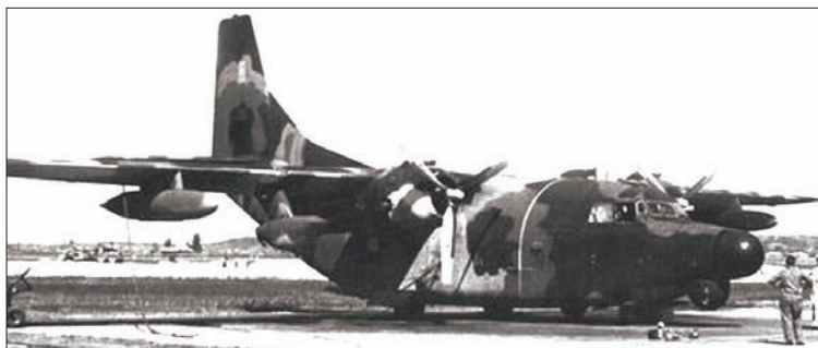
A rare image of one of the two AC-123K Black Spot aircraft, each equipped to drop up to 6,500 cluster bomblets through 12 chutes in the lower fuselage.
