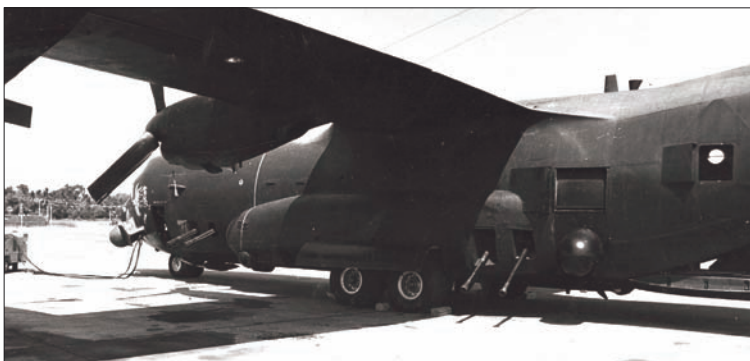
The AC-130A Surprise Package was one of the earlier gunship conversions, armed with rotary miniguns, M61 rotary 20 mm cannon, and a pair of Bofors 40 mm cannon.
