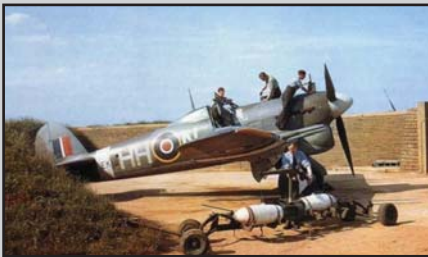
The RAF's initial policy of arming fighters with eight .303 calibre machine guns soon gave way to armament dominated by the Hispano 20 mm gun. The first fighter to use an all cannon armament was the Typhoon I, soon followed by the Tempest V. The much heavier Beaufighters and Mosquitos were armed very early with the Hispano.
