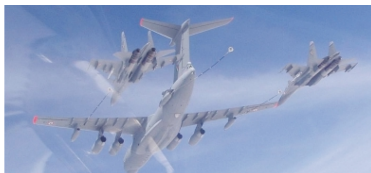
The latest addition to the IAF inventory are the first batch of Ilyushin Il-78MKI Midas tankers, each equipped with three UPAZ hose/drogue pods (IAF).
