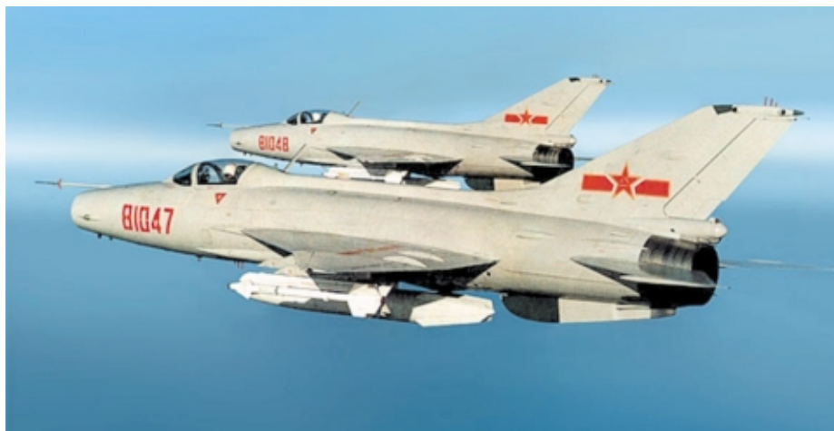
China continues to manufacture the legacy J-7, a reversed engineered and evolved Fishbed. The latest J-7E and J-7G variants employ a new double delta wing (PLA).
