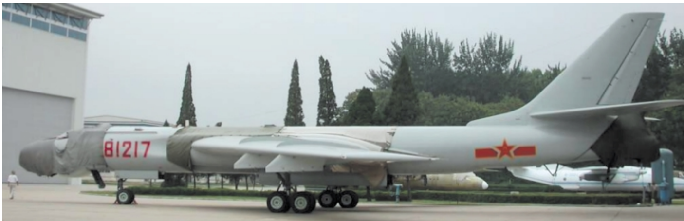
The latest photo from the Xian factory shows a H-6 cruise missile carrier, fresh from a rebuild and sporting the new low visibility grey camouflage, but full colour insignia. The upgrade includes removal of all gun turrets and the aft gunner's blisters, to save weight and reduce drag. Four pylons for 3,000 lb weight class cruise missiles replace the paired 6,000 lb rated pylons used for the YJ-6/61/62 Kraken ASMs. It is unclear whether the bomb bay fuel tank devised for the H-6U is used to further improve combat radius over gains produced by drag/weight reduction (via RD Fisher).
