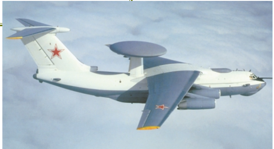
India has recently signed for the A-50I, a derivative of the Beriev A-50U/E, but equipped with the Israeli Elta L-band phased array previously bid for Australia's Wedgetail program (Beriev).
