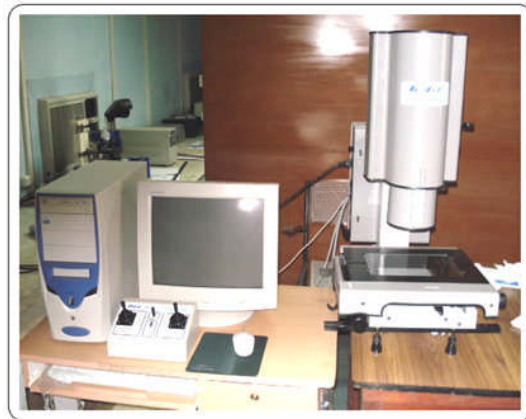
Fig. 9: Rapid 1 Computer vision system for acquiring the images.
