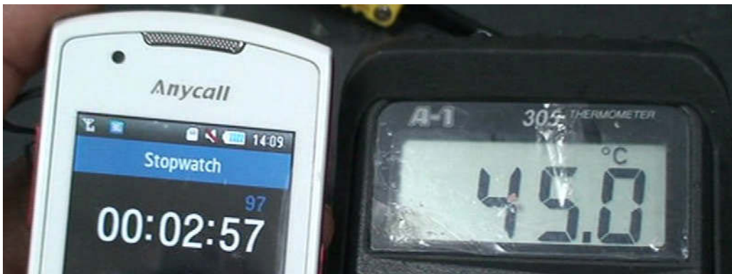
Fig. 11: Temperature measurement during the experiment (solidification point).
