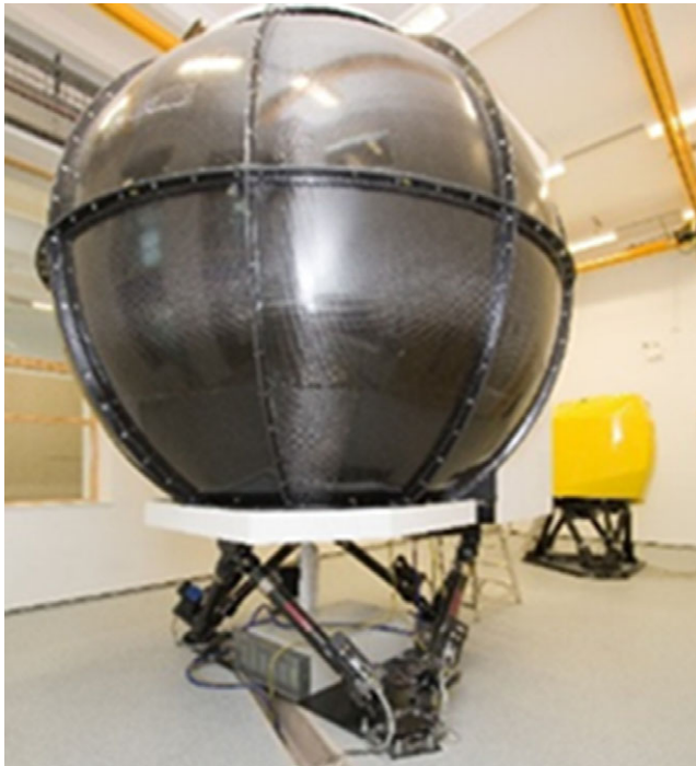
Figure 3. HELIFLIGHT-R Simulator (foreground) [27].
