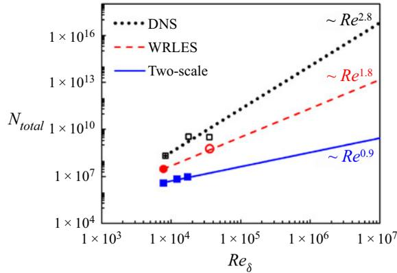
Figure 32. Mesh count– $Re$  scaling. DNS (black dots); wall-resolved LES (red dashed line); the present two-scale method (blue solid line). The open black square and red circle are for the actual  $N_{total}$ , as reviewed in Deck *et al.* (2014). Solid red circle is for the full WRLES used in the present case study (§ 2); solid blue squares are for the present two-scale calculations (§ 3).
