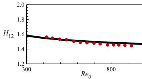
Figure 4. Shape factor  $H_{12}$  as functions of  $Re_\theta$  compared with fitted curve as a solid black line from Monkewitz *et al.* (2007). *RFTrip-x10z7*, solid brown circles. Note that not all data are shown for clarity.
