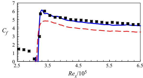
Figure 24. Friction coefficient  $C_f$  as the function of Reynolds number  $Re_x$ . The blue solid line is for the present two-scale block-spectral solution in the global coarse region. The solid black squares indicate the full LES results. The red dash line shows the ‘one-scale’ solution in the global coarse-mesh region without the source-term coupling.
