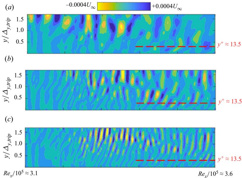
Figure 17. Dominant modes extracted from the mid  $x$ - $y$  plane from full WRLES with frequency around (a)  $St \approx 0.3$ , (b)  $St \approx 0.6$  and (c)  $St \approx 0.9$ . The blue contour colour corresponds to a negative value, while the yellow one indicates a positive value. The red dashed line indicates roughly the location of  $y^+ \approx 13.5$ , calculated with local shear velocity.
