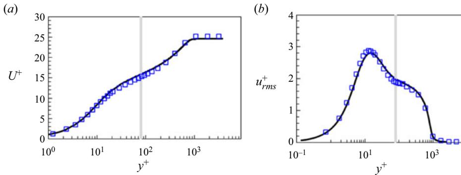
Figure 30. Mean statistics at Reynolds number  $Re_\theta \approx 2540$ : (a) mean velocity profiles and (b) streamwise velocity fluctuations with respect to the wall-normal distance. The present two-scale block-spectral solutions (open blue squares) are compared with the DNS results (Schlatter & Orlu 2010) (black solid lines). The grey lines mark the inner–outer mesh interfaces. Note that not all data points are shown for clarity.
