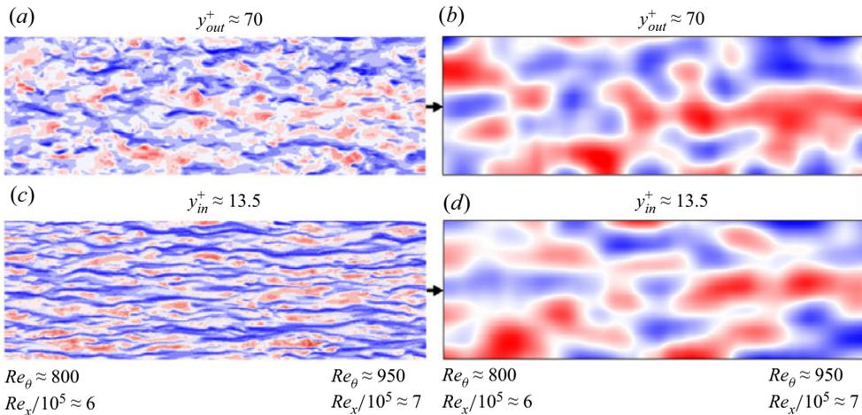
Figure 13. (a,c) Instantaneous velocity field from  $Re_\theta \approx 800$  to  $950$  at two wall-normal locations:  $y_{out}^+ \approx 70$  and  $y_{in}^+ \approx 13.5$ , respectively. (b,d) Large-scale structures retained from panels (a) and (c), respectively. The contour maximum values in panels (b) and (d) are set as  $\pm 2.4u_\tau$ .
