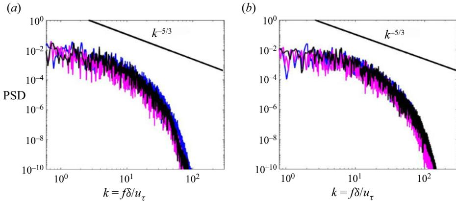
Figure 22. PSD as a function of non-dimensional frequency  $k$ : (a)  $Re_\theta \approx 600$  and (b)  $Re_\theta \approx 800$ . *Full-Span*, black lines; *Half-Span*, magenta lines; *Mini-Span*, blue lines. The energy spectra are taken at  $y^+ \sim 13.5$  as the peak energy location in [figure 21\(c,d\)](#).
