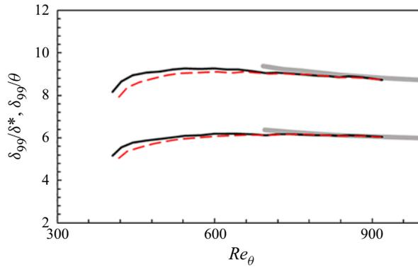
Figure 3. Indicative parameters  $\delta/\delta^*$  and  $\delta/\theta$  compared with the correlated curve of Chauhan *et al.* (2009) (solid grey lines). The present results are shown for *RFTrip-x20z7* (solid black lines) and *Base-x20z7* (dashed red lines).
