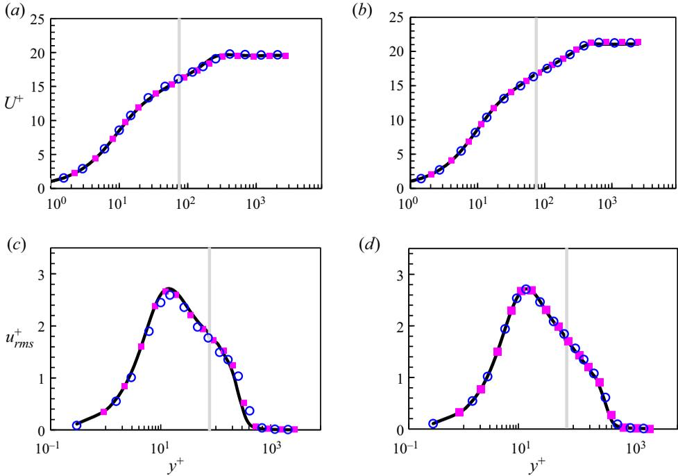
Figure 21. Mean velocity profiles as functions of wall-normal distance  $y^+$  at (a)  $Re_\theta \approx 600$  and (b)  $Re_\theta \approx 800$ . Profiles of streamwise velocity fluctuations as functions of  $y^+$  at (c)  $Re_\theta \approx 600$  and (d)  $Re_\theta \approx 800$ . *Full-Span*, solid black lines; *Half-Span*, solid magenta squares; *Mini-Span*, open blue circles. The grey lines mark the inner-outer mesh interface. Note that not all data are shown for clarity.
