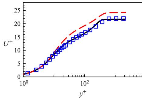
Figure 25. Mean velocity profile in relation to wall normal distance  $y^+$  in the global coarse-mesh region. The present two-scale BS solution (blue squares) is compared with the DNS result from Schlatter & Orlu (2012) (black solid lines) at the Reynolds number  $Re_\theta \approx 1000$ . The red dash line is for the ‘one-scale’ solution without the source-term coupling.
