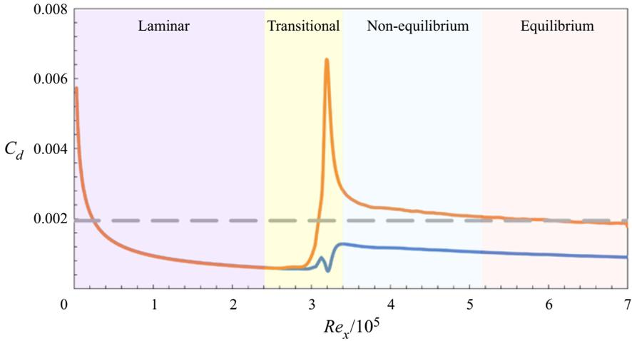
Figure 9. Dissipation coefficient  $C_d$  as functions of  $Re_x$ , categorised in four stages: laminar, transitional, non-equilibrium and equilibrium. The blue solid line depicts the viscous dissipation of the mean flow  $\epsilon$ . The orange solid line depicts the dissipation coefficient  $C_d = \epsilon + Pr$ . The grey dashed line shows the equilibrium  $C_d \approx 0.002$ .
