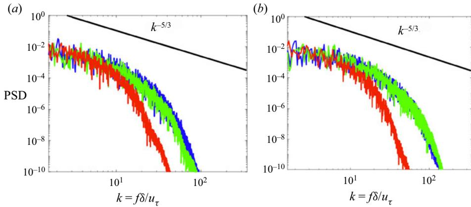
Figure 28. PSD with respect to the dimensionless frequencies. The present two-scale BS solutions (blue lines) are compared with the full LES solutions (green lines) at two Reynolds numbers: (a)  $Re_\theta \approx 600$  and (b)  $Re_\theta \approx 800$ . Red lines are for the results in the global coarse-mesh inner region. The energy spectra are taken at  $y^+ \sim 13.5$ .
