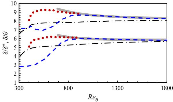
Figure 8. Indicators  $\delta/\delta^*$  and  $\delta/\theta$  compared with the experimentally correlated curve of Chauhan *et al.* (2009) (solid grey lines). The results of the tuned ‘optimal’ tripping of Schlatter & Orlu (2012) (‘OP-KTH’) are shown as dash-dotted black lines; the natural TS-wave transitions (‘TS’) are shown as dashed blue lines; the present calculations (RFTrip-x10z7) are shown as solid brown circles.
