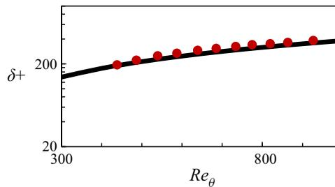
Figure 5. Boundary layer thickness  $\delta^+$  as functions of  $Re_\theta$  compared with the fitted curve as a solid black line of Schlatter & Orlu (2010). *RFTrip-x10z7*, solid brown circles. Note that not all data are shown for clarity.
