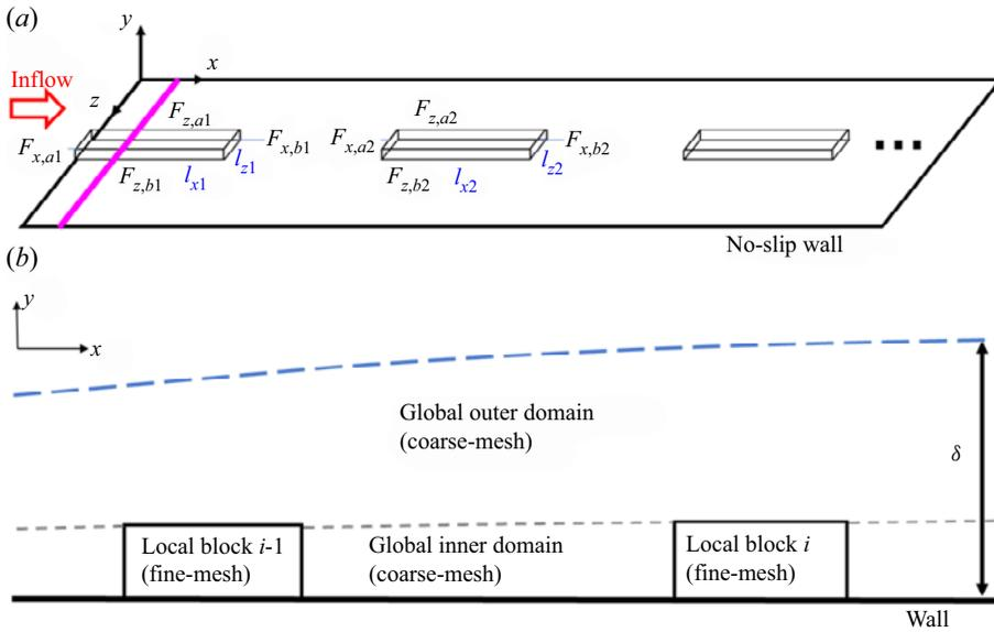
Figure 18. Illustration of computational domain with the near-wall embedded DNS blocks. (a) Overall view of the configuration (the solid magenta line indicates the trip). (b) Close-up  $x$ - $y$  cut plane view.
