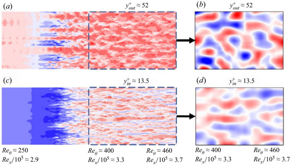
Figure 12. (a,c) Instantaneous velocities on cut planes at two wall-normal locations:  $y_{out}^+ \approx 52$  and  $y_{in}^+ \approx 13.5$ , respectively. (b,d) Corresponding large-scale structures retained from the regions marked by black dashed boxes in panels (a) and (c), respectively. The contour maximum values in panels (b) and (d) are set as  $\pm 2.74u_\tau$ .
