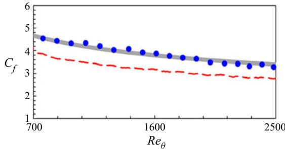
Figure 29. Friction coefficient  $C_f$  as a function of Reynolds number  $Re_\theta$ . The solid grey lines indicate the correlated curve by Smits *et al.* (1983). The solid blue circles are for the present two-scale BS solution. The red dashed lines are for the one-scale solution without the source-term coupling. Both results are taken from the global coarse-mesh region. Note that not all data points are shown for clarity.
