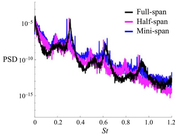
Figure 20. Turbulence power spectra density (PSD) with respect to the non-dimensional frequency, Strouhal number  $St$ . The black, magenta and blue lines are for the *Full-Span*, the *Half-Span* and the *Mini-Span* results, respectively.
