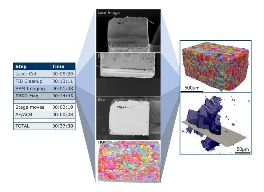
**Figure 1.** From data collection to volumetric analysis and defect identification. TriBeam experiment steps and approximate durations (left), various data modalities collected (center), 3D reconstructions of the bulk and a defect (right).
