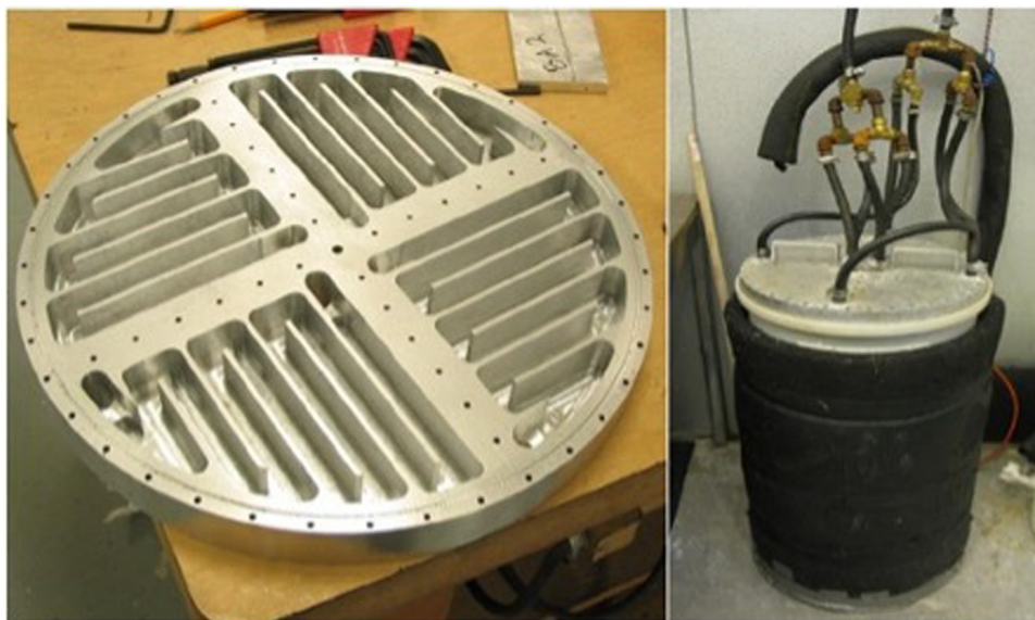
Fig. 1. Cold plate used for controlled cooling in direct contact with the solution sea ice (Schulson and others, 2015).
