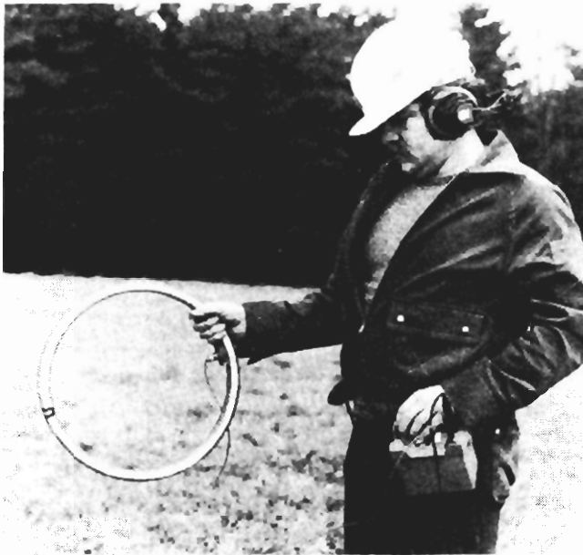
Fig. 34. Surface receiver for detection of trapped miners.
