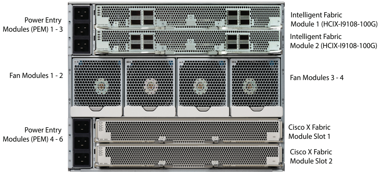
Figure 3 Cisco Compute Hyperconverged 9508 Chassis Rear View with HCIX-I9108-100G (top) and 2 Fabric Module Slots (bottom)
