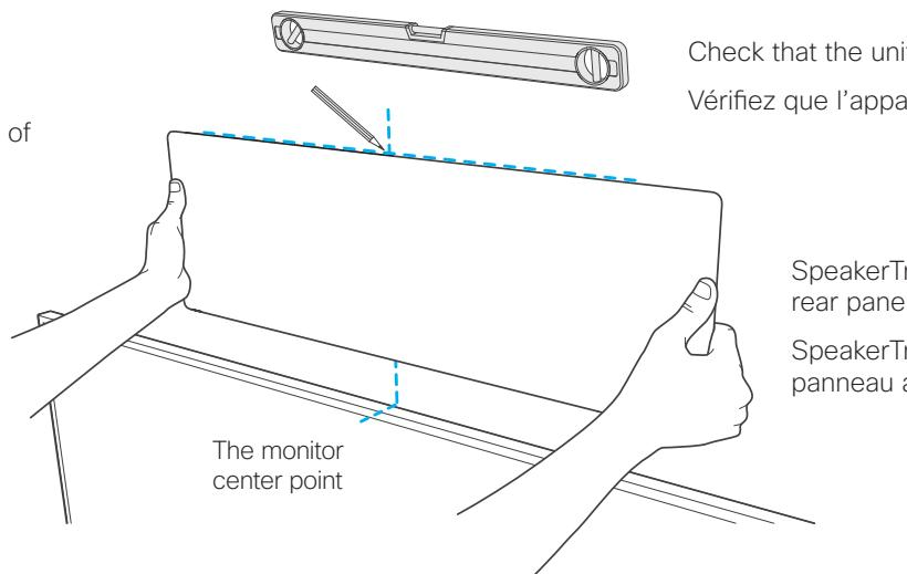
Use the template on the other side of this sheet when drilling holes for the wall bracket. Screw dimension M6.
