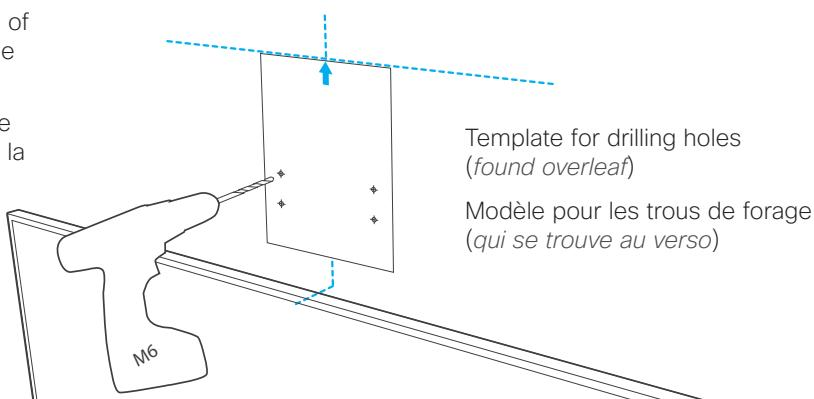
Select the type of attachment for the wall bracket on the basis of the type of material the wall is made of (wood, concrete, gypsum).
