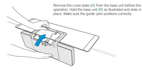
Use the four pan headed screws (P) when fastening the base unit. Use the Torx Key (M) and tighten the screws.
