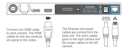
Start with the camera to the right and hold the camera as illustrated. Make sure the short cables (Ethernet and power) are available for this camera and connect the cables. Then connect the HDMI cable coming from the codec. Guide the camera into position.
