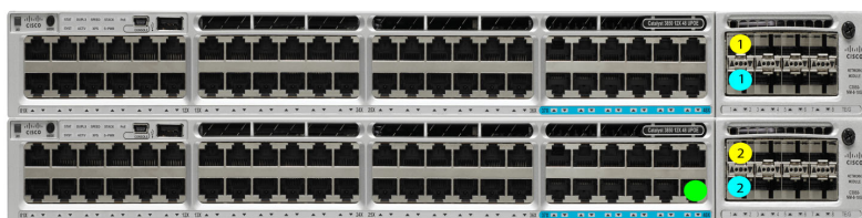
Dual 10/25GE ToR Switches (standalone or stacked)
