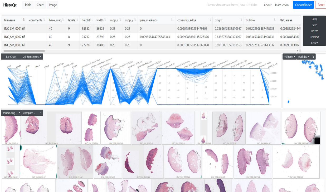
Figure 17: The output of the HistoQC tool for the INCLIVA dataset. The euclidean plot helps in identifying outliers with a variation in the dataset. WSI can be sort by “flat_areas” to find higher tissue presence on the slide. Pen markings can be quickly evaluated by sorting with higher values or with “tenenGrad” to find faded slides.
