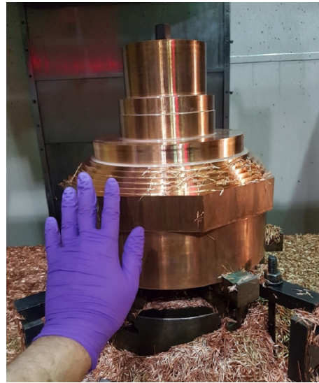
(b) Main cavity bell partially milled.
