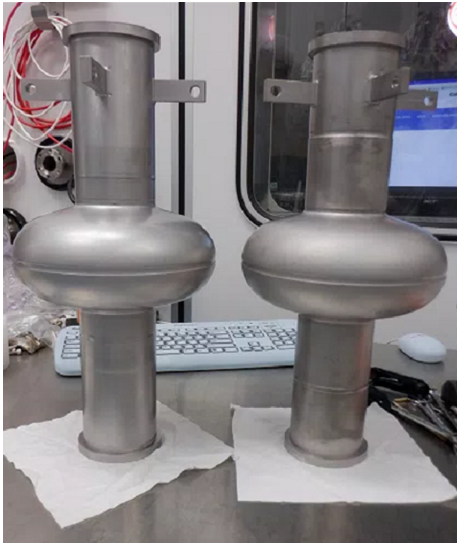
Figure 11.2: Left: The new Nb 3 Sn cavity. Right: A standard coating Nb 3 Sn cavity. Note that the new cavity is shinier suggesting a smoother surface.
