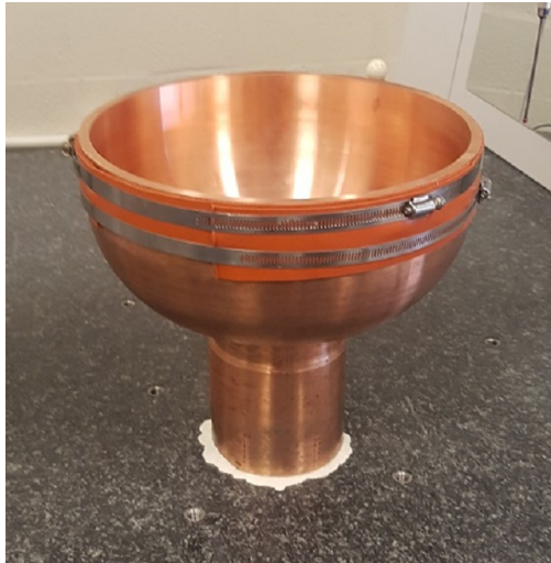
(c) Complete copper bell being indexed to confirm the shape.
