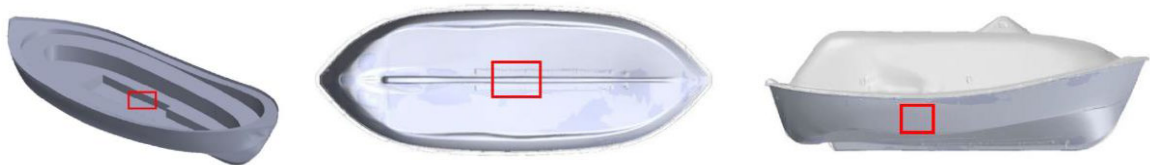
Figure 22: Sampling locations for fractographic analysis. Credit: DNV-GL.
