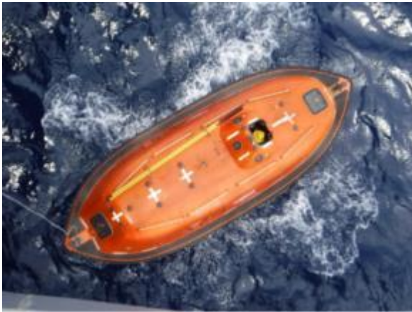
Figure 4: Lifeboat No. 6 in water but still hooked up to fall cables. Credit: Palfinger, dated 2015.
