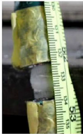
Figure 60 (far left) and 61 (right): The white polyethylene liner evidencing forces of compression and stretching after the wire layer is fully compromised. These photos were taken during the Coast Guard's experiment at MSTC. Credit: CG.
