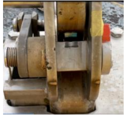
Figure 6: The “flat face” of the locking shaft on a LHR 3.5M2 hook (image does not depict Lifeboat No. 6’s hook). Credit: CG.
