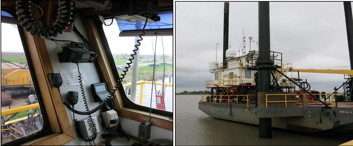
Left picture shows view towards the starboard bow of B.W. Haley as seen from captain's wheelhouse conning position. Right picture shows radar shadow area to wheelhouse of B.W. Haley .
