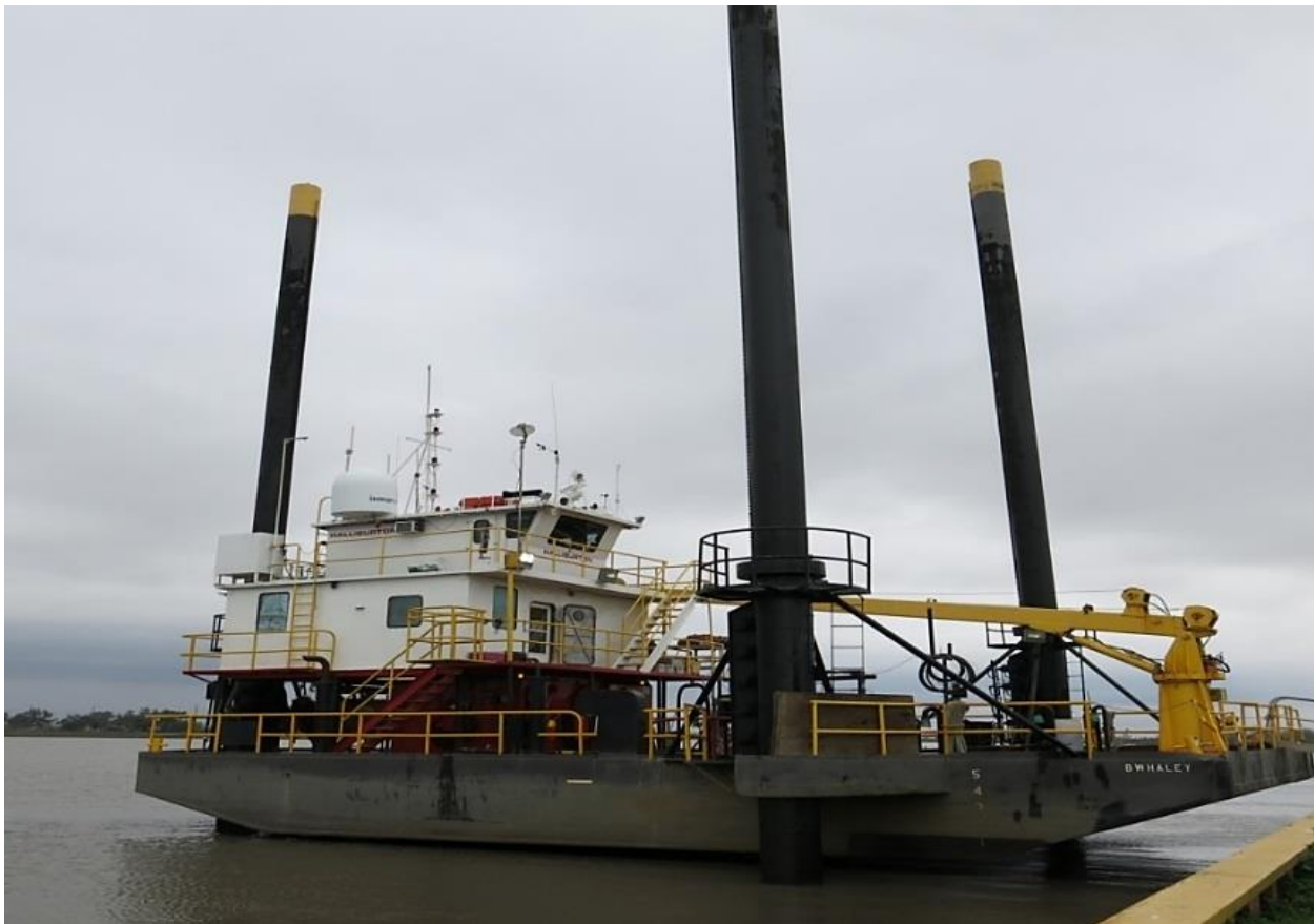
Liftboat B.W. Haley with legs in “elevated” position.
