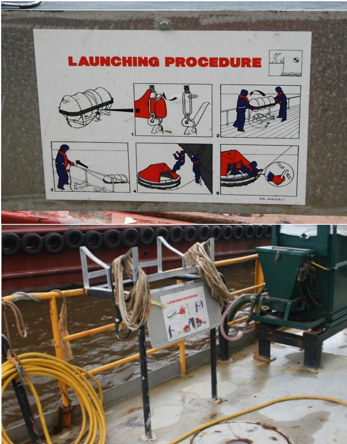
Figure 6. The illustrations, posted below the liferaft cradles, showing how to launch the liferafts.
