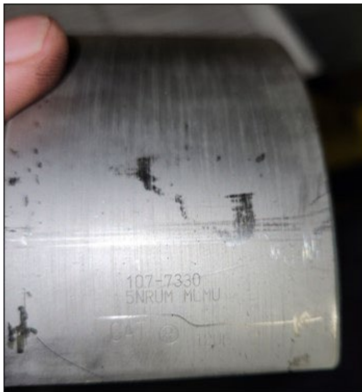
Figure 6. Part number on a typical Caterpillar main bearing. (Source: Stabbert Maritime)
