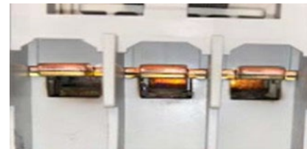
Figure 2: Welded contactors (Image courtesy of Chevron North America)
