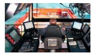
The DP operator station should display information from the power system, thruster system and control system to ensure that these systems are functioning correctly. Information necessary to safely operate the DP system should be visible at all times. Other information should be available upon the operator's request.
