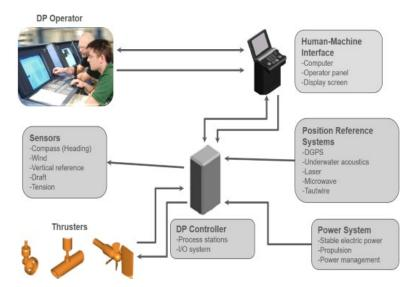
The DP System maintains a vessel's desired position and/or heading by use of the DP control computer which automates the control of vital power and propulsion systems in order to control 3 of 6 axes of a vessel's movement:
