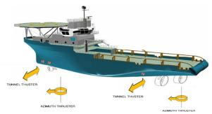
The thruster system shall be arranged as to provide the vessel with adequate maneuverability under all operating conditions. Also, the thruster system should be able to provide adequate thrust to control surge, sway and yawing.
