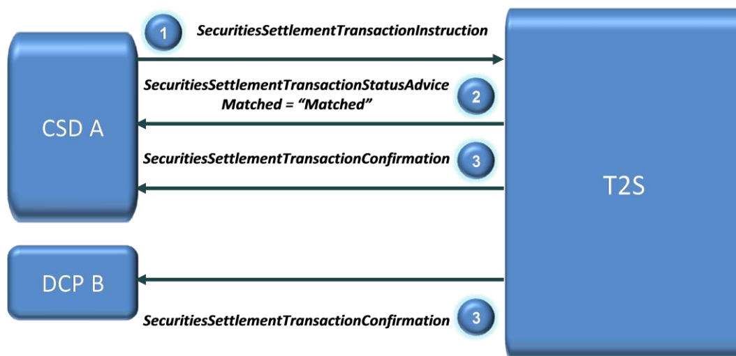
DIAGRAM 16 - MESSAGE FLOWS EXCHANGED BETWEEN THE T2S ACTORS AND T2S (A)
