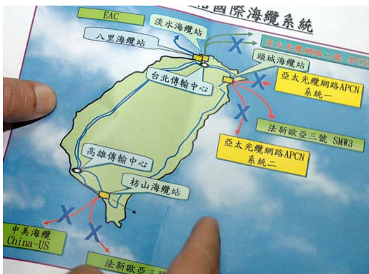
Fig. 25 The damage status of 5 undersea optic-fiber cables
