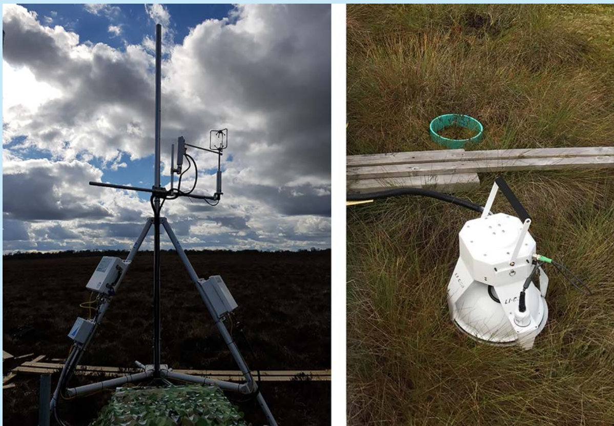
Figure SB6.1. Eddy covariance tower and portable chamber system used to measure carbon and greenhouse gas dynamics from Clara bog, Co. Offaly. Photo: M. Saunders and R. Ingle.
