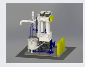
The produced process gas is stripped of the remaining by-products through a process of gas purification. Here, a combination of wet gas scrubbing and cooling filters the gas.
