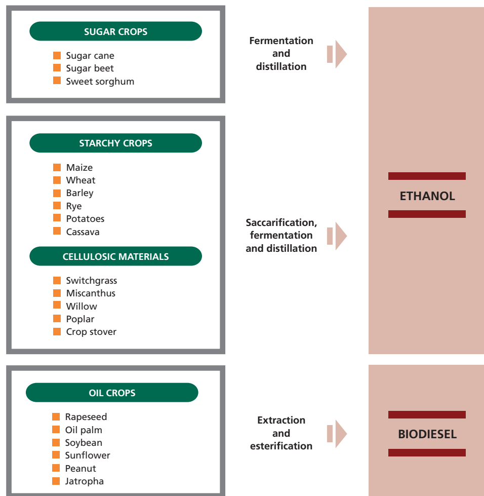
FIGURE 6 Conversion of agricultural feedstocks into liquid biofuels
