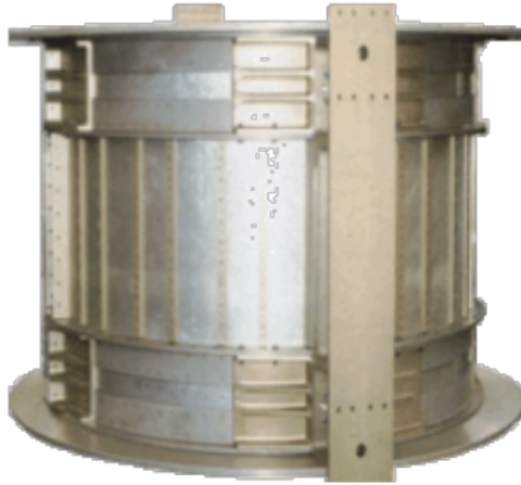
Figure 2.3: The AMS-02 permanent magnet. The magnet has flown in space during the AMS-01 mission in '98 [49]
