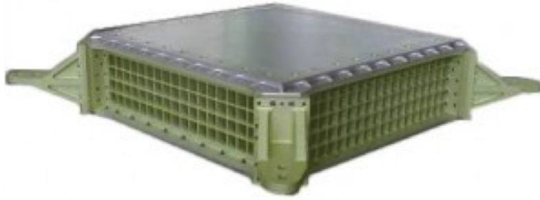
Figure 2.18: Mechanical structure of ECAL not yet instrumented with the PMTs. Each square guide on the sides is designed to host a single PMT.
