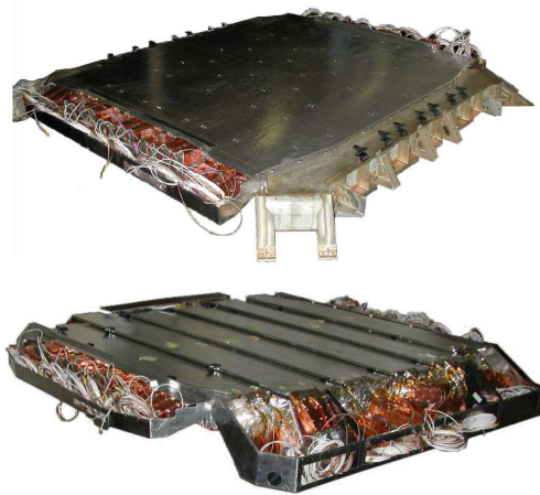
FIGURE 2.7: The completed upper and lower ToF before the final shielding. The scintillator paddles, the bent light guides and the PMT are exposed.
