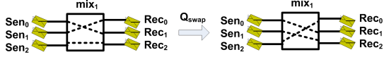
Figure 5: Q_{\text{swap}} transition operation on the second and third links of a mix
