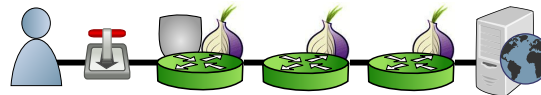
Figure 2: Throttling occurs at the connection between the client and guard to capture all streams to various destinations.
