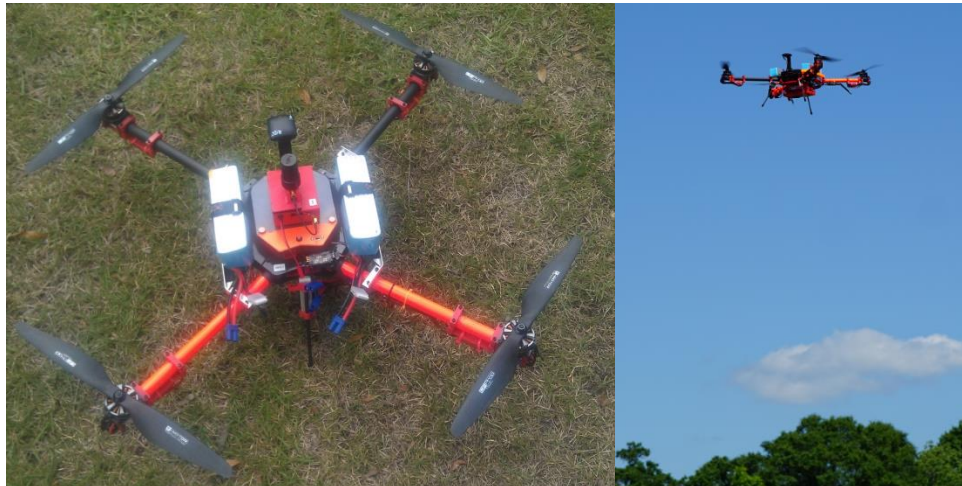
Figure 5.2.3.2.1 MAP-M4 VTOL Multirotor UAS vehicle
