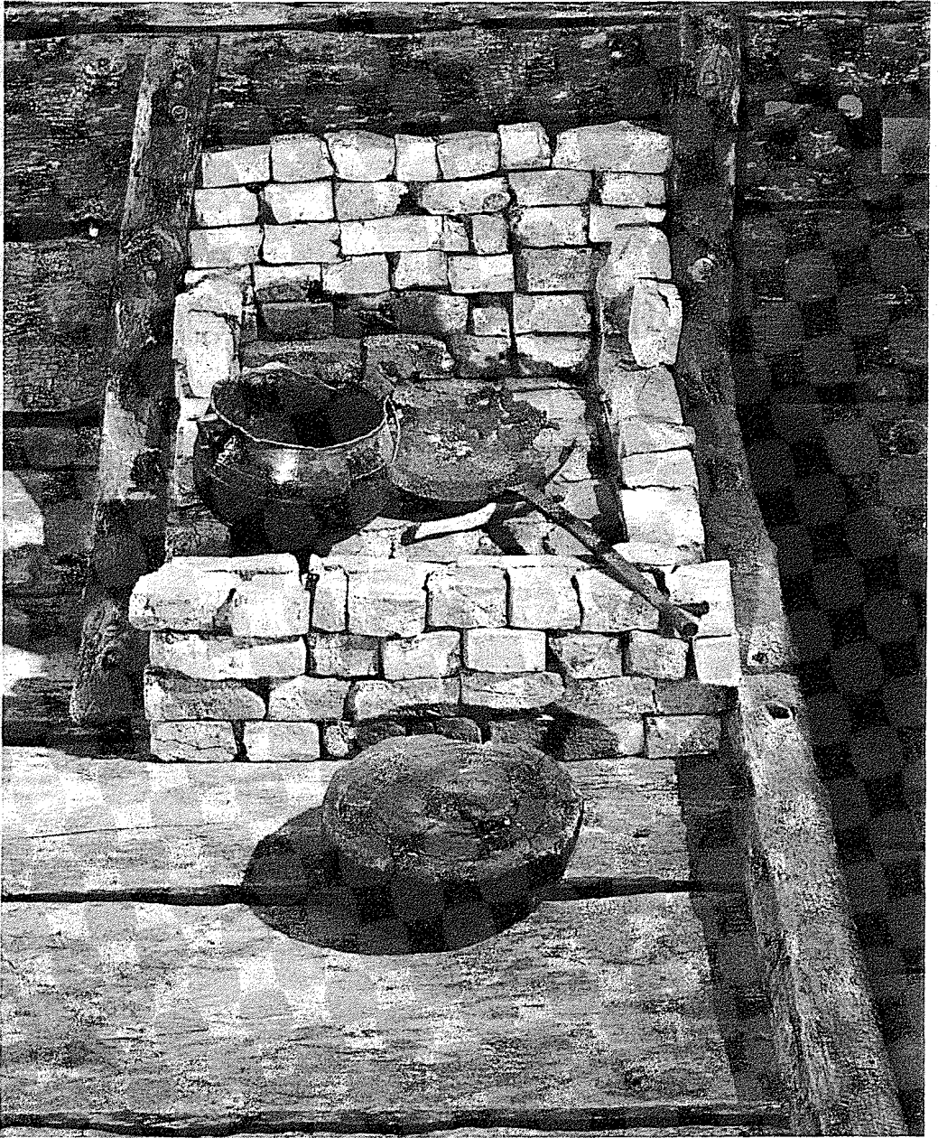
Brick hearth on board a small American armed vessel of the Revolutionary period.
