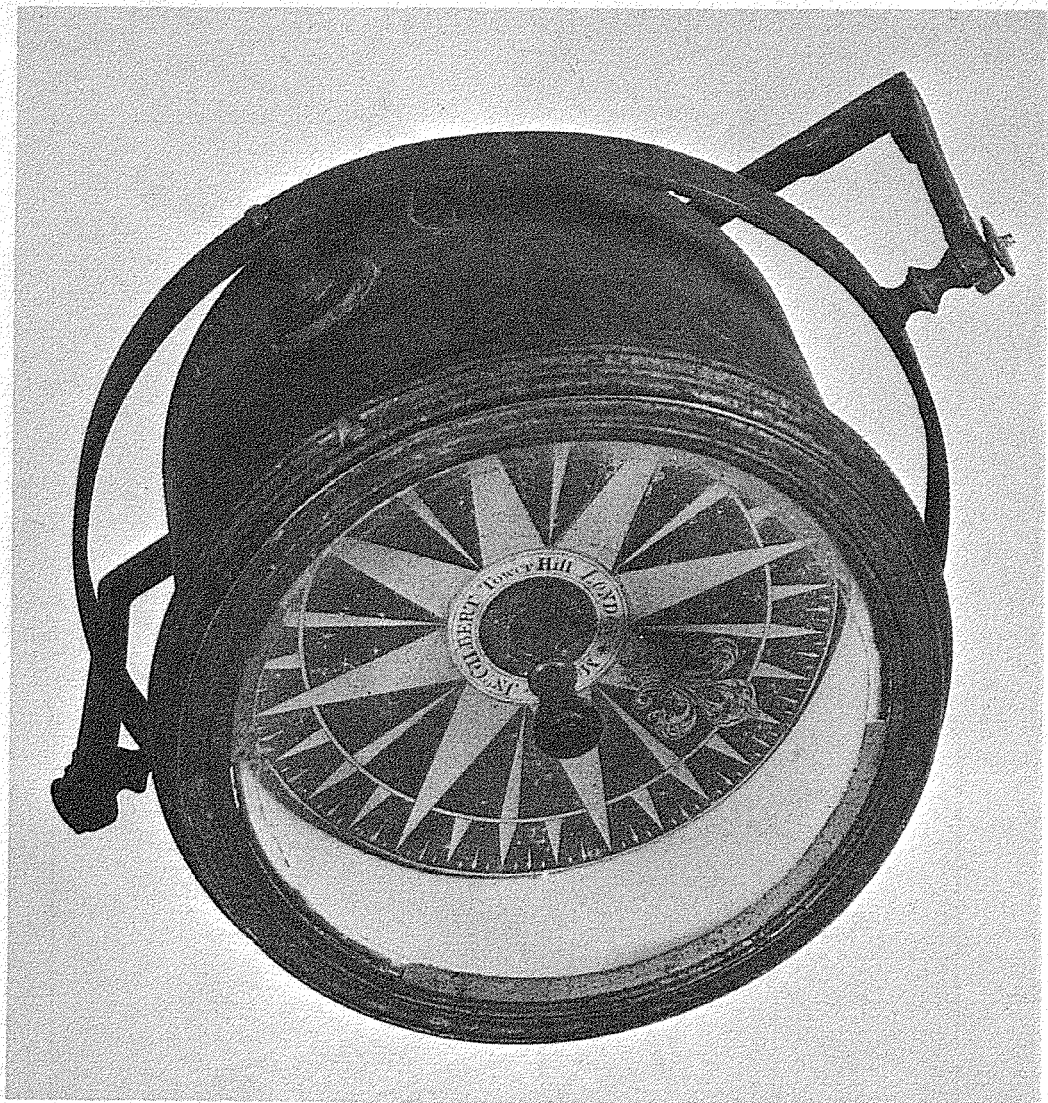
XII. Hanging Compass, the brass case "Made by Jno Gilbert Tower Hill, London."
