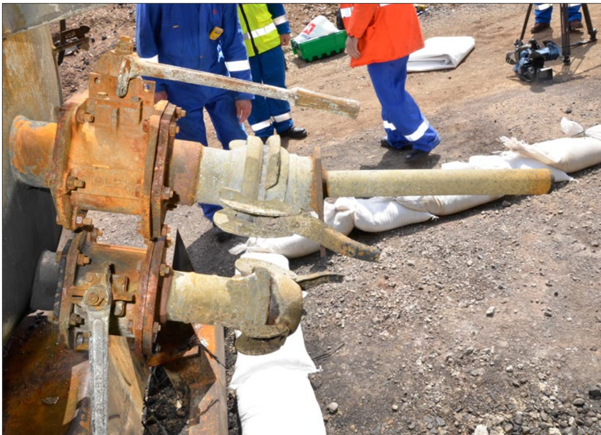
Figure 10 Two-inch inlet adapter on rear of vacuum tanker
