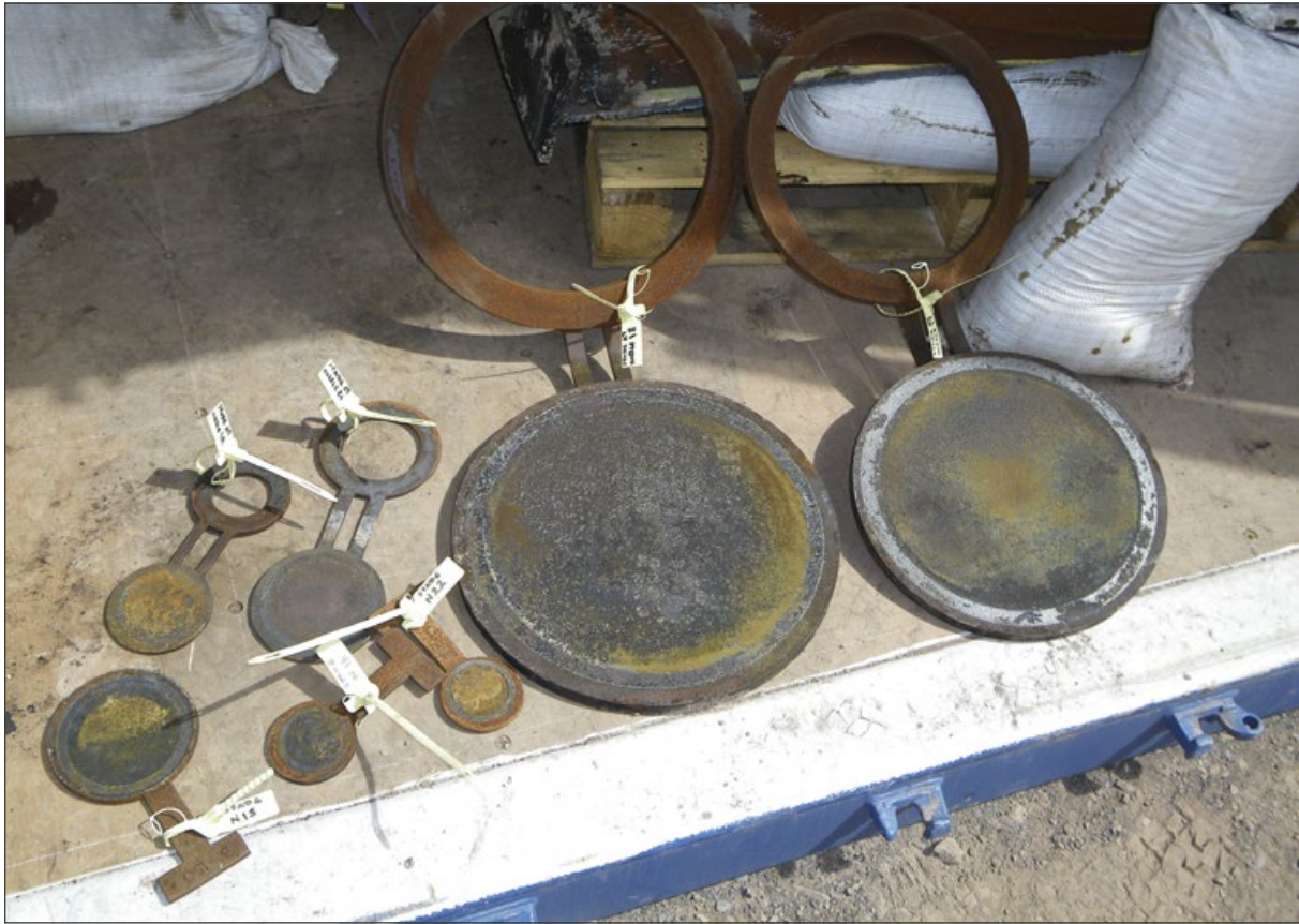
Figure 9 Photograph of isolation spades and blinds from tank 17T302
