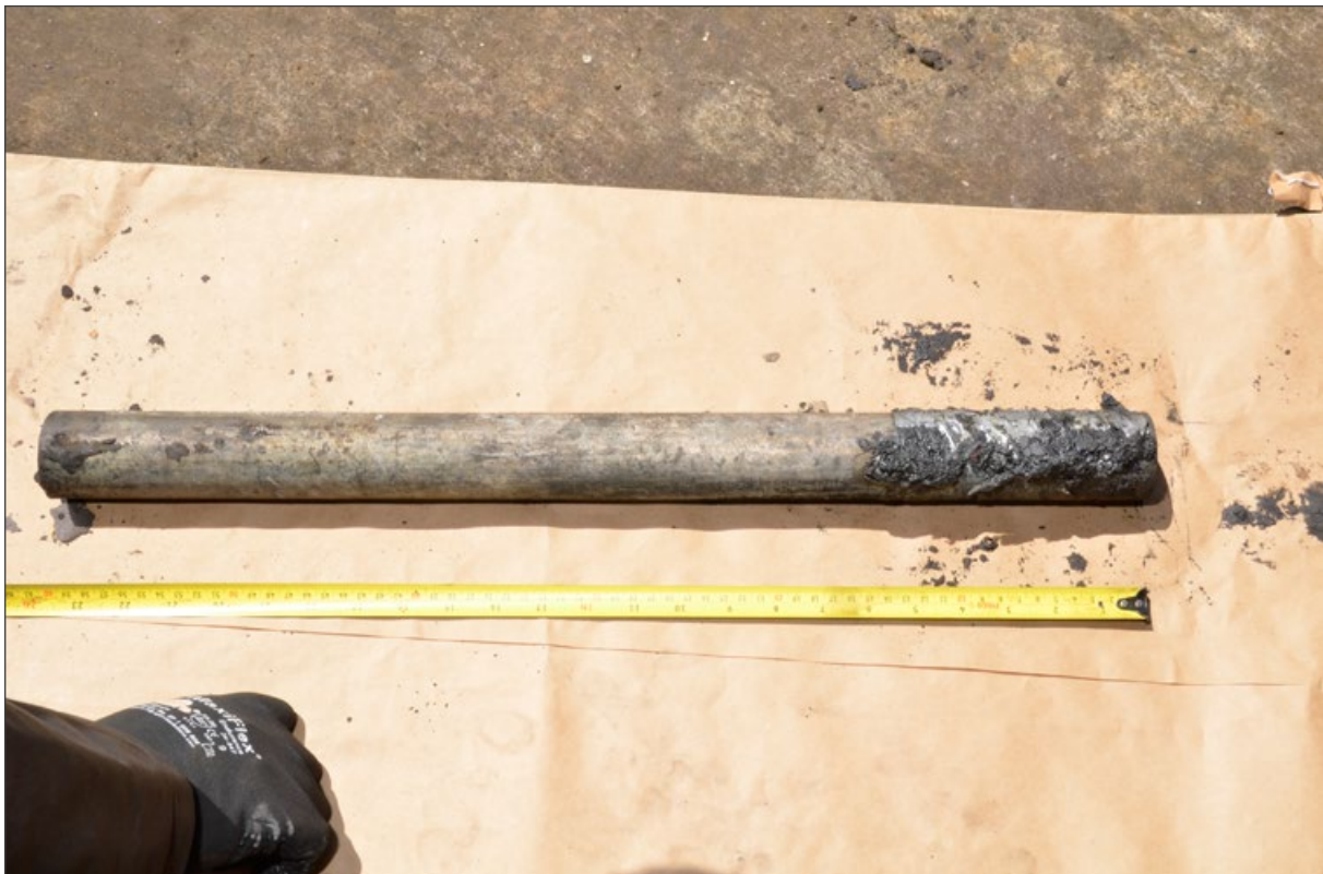
Figure 14 Photograph of scaffold pole found within tank 17T302
