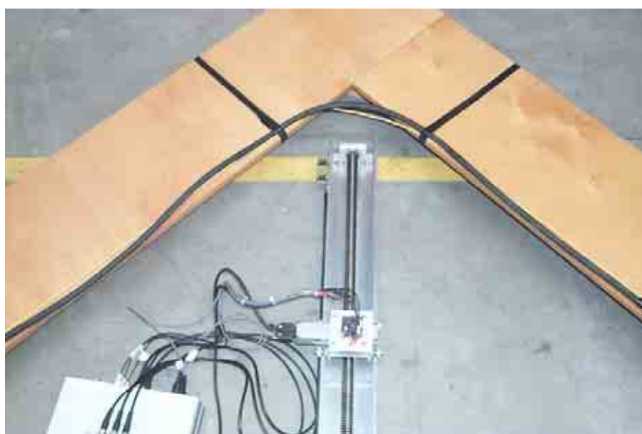
Figure 4 Measurements on arc welding cable
