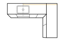
**3** It's important to indicate the location of the sink. Measure from the corner of the countertop to the center of the base cabinet where your sink is located.
