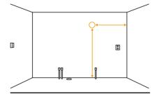
**6** Measure ventilation outlet for kitchen exhaust hood.
