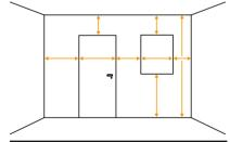
**4** Measure each wall fully from floor to ceiling and from doors to windows. Remember to include door and window frames.
