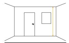
**3** Measure the floor to ceiling, marking the highest and lowest points. Remember to include soffits.
