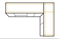
2 Measure your countertop starting from one corner to the opposite end. Make sure that all length and depth measurements are taken from at least two places. Don't forget to add 1½" to account for overhang.
