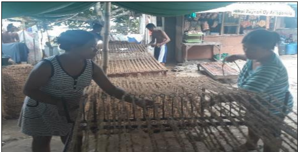
Figure 13. Village-level weaving of geonets at Tropical Prime Coir Corp., Padre Burgos, Quezon.
