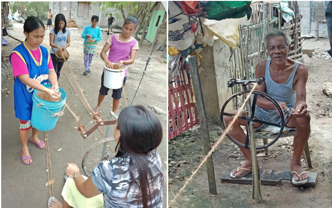
Figure 12. Village-level twining of cococoir of Tropical Prime Coir Corp. at Unisan, Quezon.
