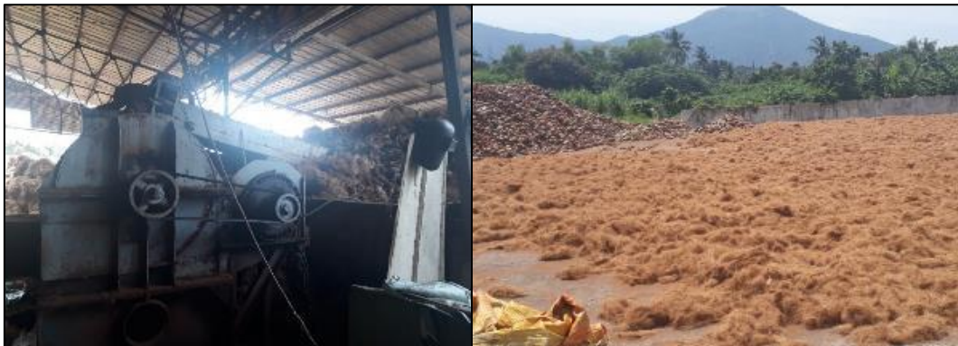
Figure 10. Decorticating machine and solar drying of coco coir at Wua Yei Enterprises in Victoria, Laguna.
