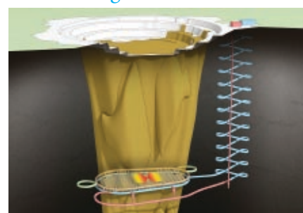
Access Development and Start of Production Drift Development
