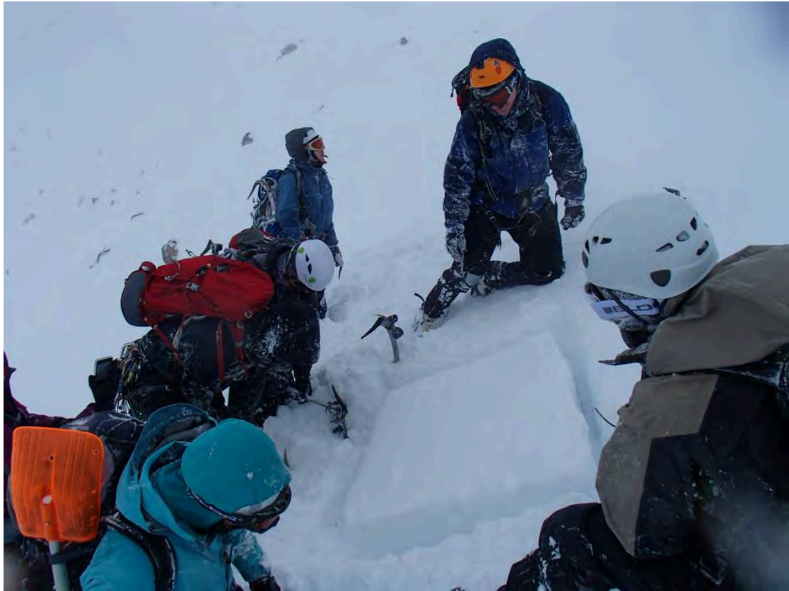
Avalanche block test. The layer of fresh snow slid off the old snow in a textbook windslab avalanche.
