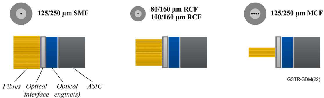
Figure 3 – Optical interface density achieved with regular single-mode fibre, RCF and MCF
