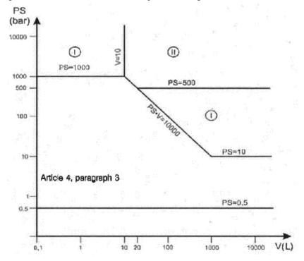
(ii) Exceptionally, assemblies intended for generating warm water at temperatures not greater than 110°C which are manually fed with solid fuels and have a PS.V, shall be subject either to a Type examination (Module B — design type) with respect to their conformity with the essential requirements referred to in paragraphs 14, 15, 16, 17 and 30 and subparagraphs 33(2)(a) and (d) of Schedule 2 to these Regulations, or to full quality assurance (Module H).
